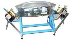
TQC have designed and manufactured a number of bumper punch systems varying in complexity.
